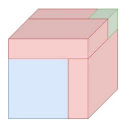
Let u be the length of the side of the large cube that is formed by the blue cube, the red boxes, and the green cube. Let v = u - y. Now, the green cube has side v and the blue cube has side y. The three red rectangular boxes have sides with lengths u, v, and y, and the big cube that is formed by all the other shapes has side length u.
